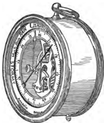
FIG. 66. AN ANEROID BAROMETER (A BAROMETER WITHOUT QUICKSILVER)
